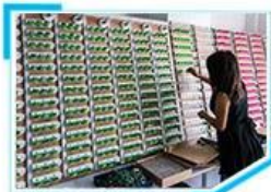
9. Aging test for travel charger
